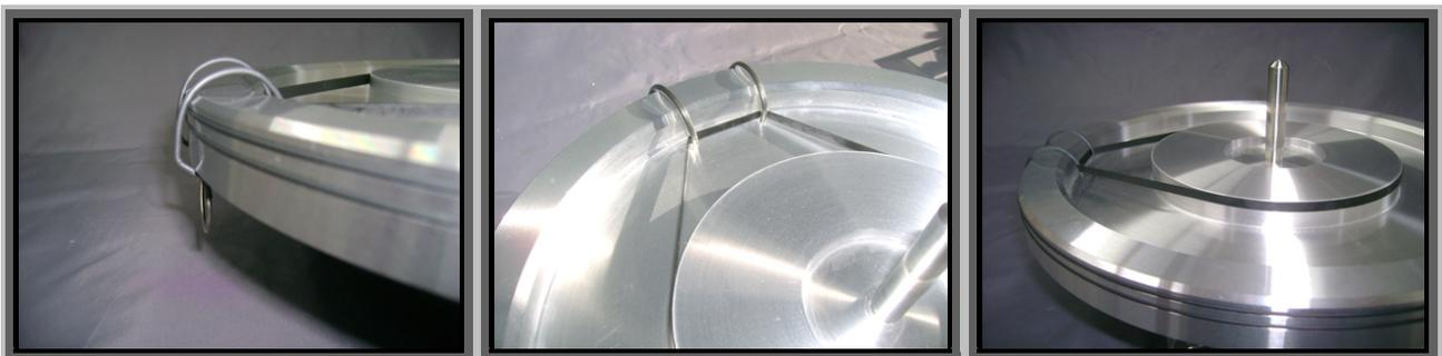
**Explanation ...** If the drive belt remains at the bottom of the platter around the inner hub there will be a misalignment with the height of the motor pulley. When the platter starts rotating the drive belt will then jump out of the motor pulley.
