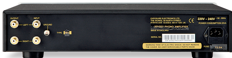
ABOVE: The rear panel of the 3010S2 Phono Stage continues the theme of simplicity with only input and output connections, an earthing post and IEC mains inlet to be seen. Different PCBs are available for MM/MC matching
