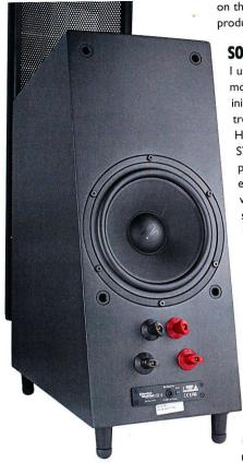
The rear carries an 8in lowbass unit, bi-wire inputs that allow XStat panel and bass bin to be electrically split, and a small 15V d.c. supply input socket, with blue LED indicator to confirm power. A rear grille is supplied.
